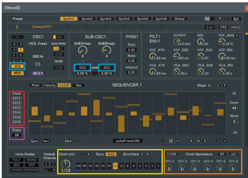
Any sequencer (1-6) can be step-triggered by *any* clock divider (1-6) by activating the necessary [Clock-DIVx] toggles (highlighted in red, in the picture above), at the individual sequencer level. Result: if a [Clock-DIVx] toggle is enabled, then the clock division from *that* divider is sent to *that* sequencer.
