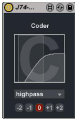
Note: the All-in-one audio device contains internally the same vocoder as the VoCoder separated device, with filter and octave parameters being fixed (to high-pass mode and default settings).
